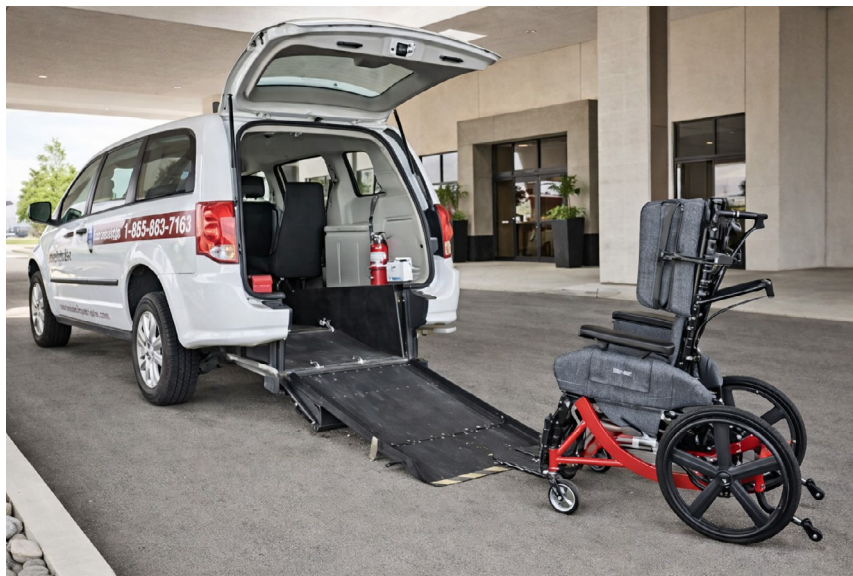
Fig. 6. Vehicle adapted for persons with mobility disabilities (with ramp)
