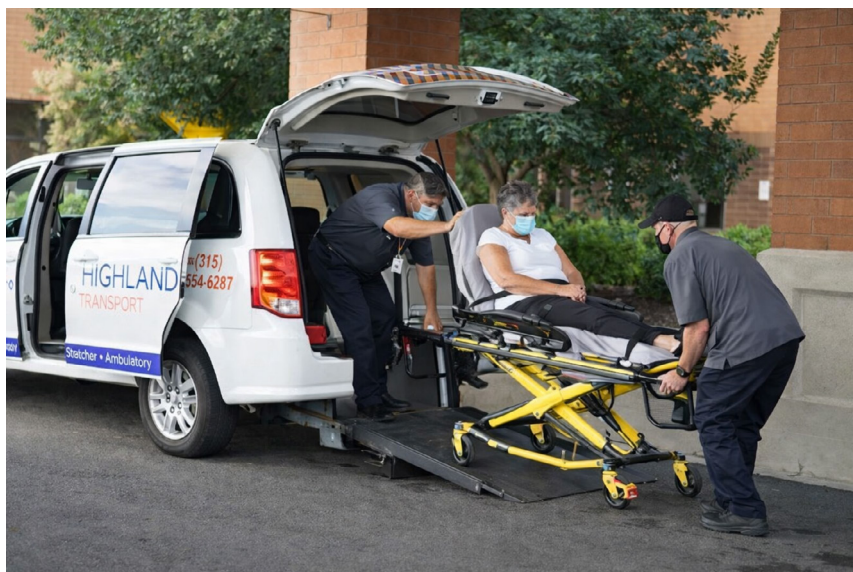
Fig. 7. Vehicle adapted for transporting persons in a lying position (with ramp)
